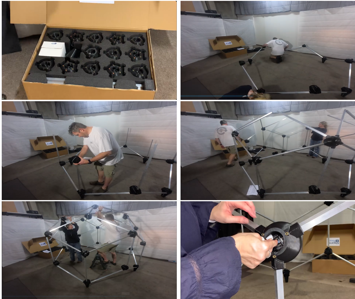
Figure 4 Stages of construction over a time of around 40 minutes for a 1800mm array. Additional time is required for running cables through the interior of the frame. A reasonable estimate of time for setup would be 2-3 hours.
